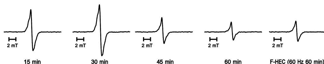
Fig. 2-7 Observed time-course ESR spectra of fractured polymers at 60 Hz.
