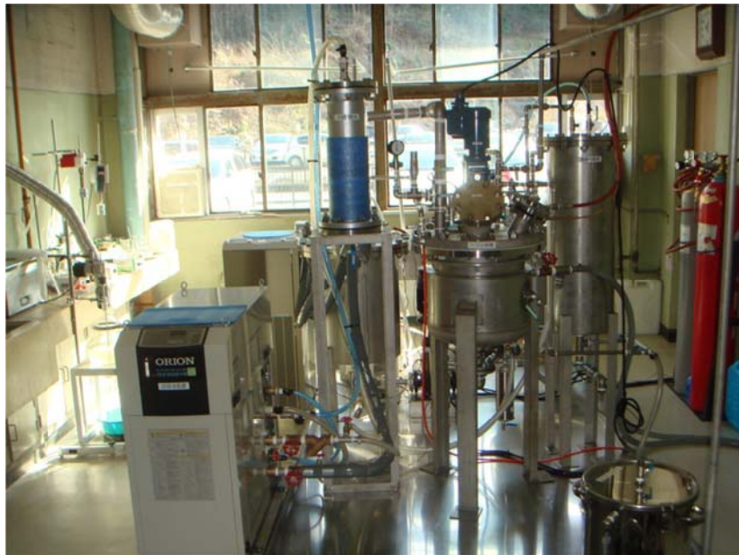
Figure 2-5. Continuous pilot plant for the degradation of PCBs under mild conditions
