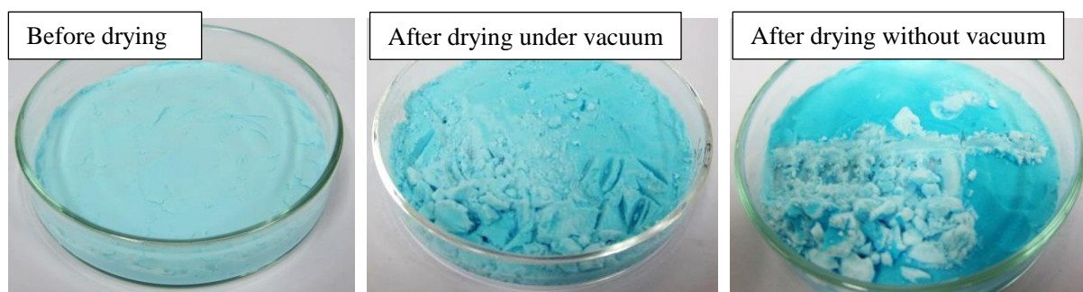
Fig. 2-1 Images of BB solution absorbed FR before and after drying with/without vacuum.
