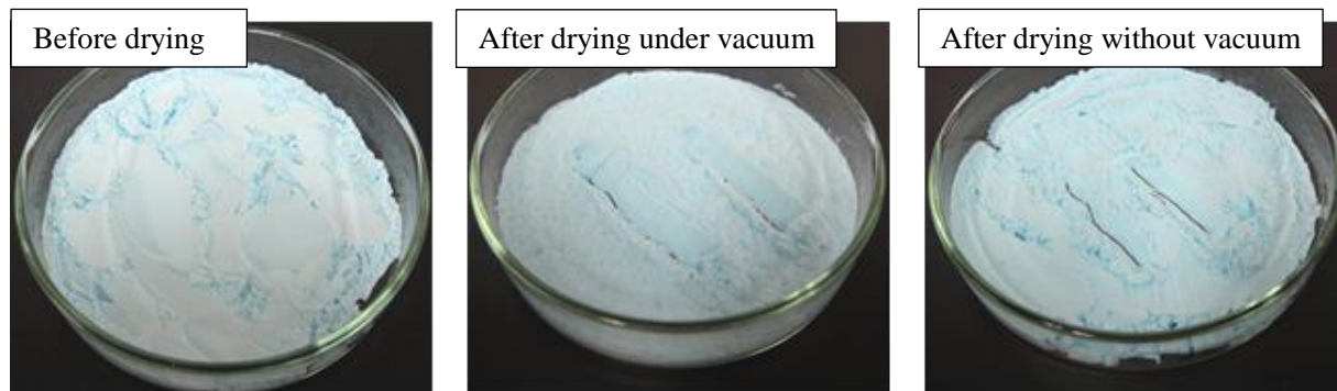
Fig. 2-2 Images of BB ethanol solution absorbed FR before and after drying with/without vacuum.
